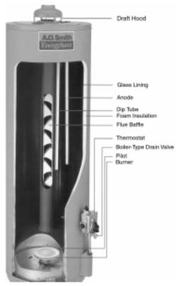
**Control:** There is one control on this style of water heater. The control has a main gas regulator, pilot gas regulator, on-off-pilot knob, controls water temperature, has a temperature adjustment knob, and a high water temperature limit safety.
